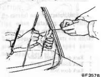
Fig. BF-64 Cutting Sealant
