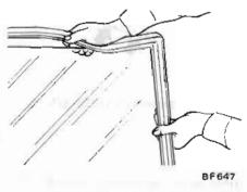
Fig. BF-84 Installing Weatherstrip
