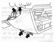
Fig. BF-91 Removing Instrument
