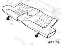
Fig. BF-98 Removing Seat Cushion
