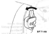
Fig. BF-99 Unlocking Lock Knob
