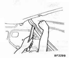
Fig. BF-83 Removing Back Door Weatherstrip
