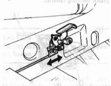
BF693B Fig. BF-59 Adjusting Front Clamp
