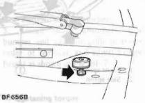
Fig. BF-19 Loosening Hood Bumper Height Nuts
