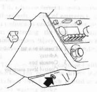
BF7058 Fig. BF-90 Removing Instrument Console Bracket Cover
