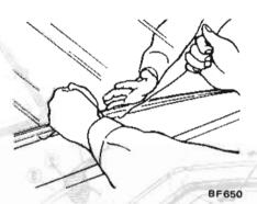
Fig. BF-86 Fitting Weatherstrip (Bottom)
