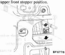
Fig. BF-43 Adjusting Upper Front Stopper
