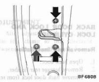
Fig. BF-46 Removing Door Lock
