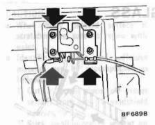
Fig. BF-55 Removing Back Door Lock
