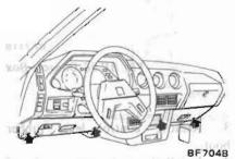
Fig. BF-89 Removing Instrument Lower Covers
