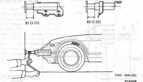
Fig. BF-9 Checking Shock Absorber Function
