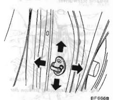
Fig. BF-29 Adjusting Door Lock
