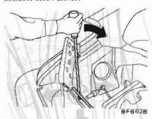
Fig. BF-25 Removing Torsion Bar
