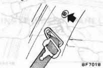
Fig. BF-81 Removing Center Pillar Finisher
