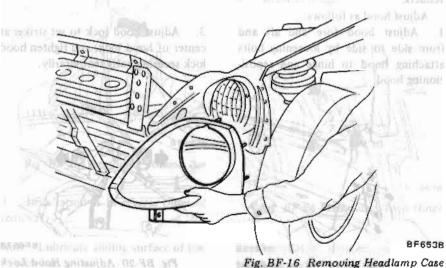
Fig. BF-16 Removing Headlamp Case
