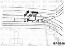
Fig. BF-50 Adjusting Back Door
