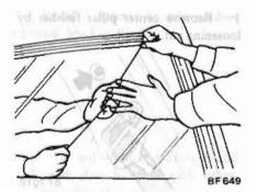
Fig. BF-87 Fitting Weatherstrip (Top)
