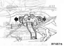
Fig. BF-20 Adjusting Hood Lock
