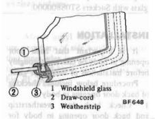
Fig. BF-85 Inserting Cord in Weatherstrip
