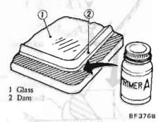
Fig. BF-69 Applying Primer A
