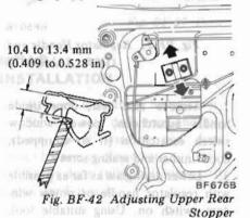
corrected and the second of th 2. Adjust front height of glass, same as rear upper stopper, by changing
