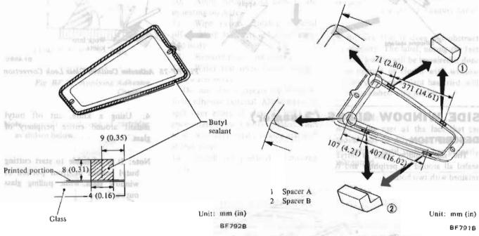
Fig. BF-78 Attaching Butyl Sealant
