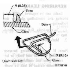
Fig. BF-68 Installing Dam Rubber
