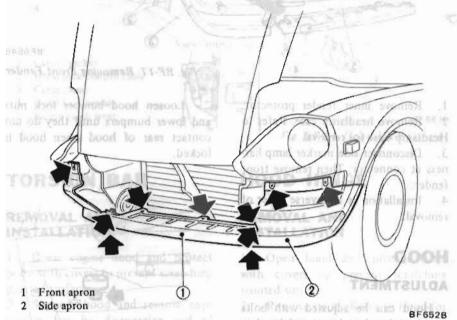
Fig. BF-15 Removing Front Apron and Side Apron
